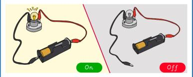
If there is a break in a series circuit, the electrical current will be cut and all the components will stop working. Causing a break in a series circuit can act as a switch to turn off the circuit off.
